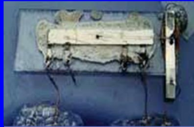
First Integrated Circuit, 1958 Jack Kilby, Texas Instruments
